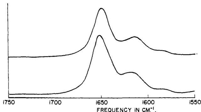
Fig. 2.—Infrared spectra of cytidine (upper curve) and deoxycytidine (lower curve) in  $\text{D}_2\text{O}$  solution, pH 7, 25- $\mu$  path length. Ordinate is absorbance on arbitrary scale.
