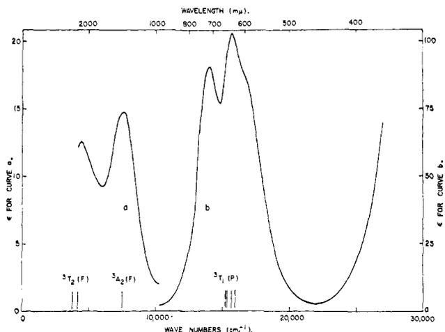
Fig. 1.—Absorption spectrum of  $\text{NiCl}_2$  dissolved in molten CsCl at 680°. The molar extinction coefficient scale for the visible spectrum, curve b, is on the right while the scale for the infrared spectrum, curve a, is on the left. Computed values of the excited-state energy levels for  $Dq = 370 \text{ cm}^{-1}$  are indicated immediately above the wave-number scale.
